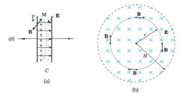
The electric field inside the plates of the capacitor is directed perpendicular to the plates. The magnetic field this gives rise to via the displacement current is along the perimeter of a circle parallel to the capacitor plates. So B and E are perpendicular in this case.
