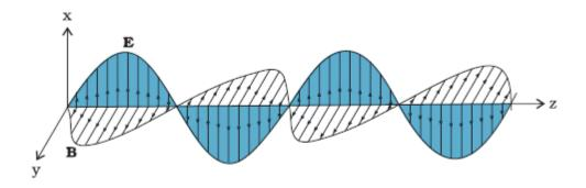
The above figure shows a typical example of a plane electromagnetic wave propagating along the z direction.
